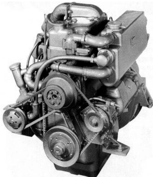
A FORD XLD-418-XLD416 marine engine fitted with combined heat exchanger header tank and water cooled exhaust manifold type FM180-3872.
